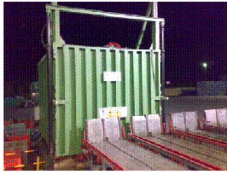
Figure 3.2. Vacuum cooling system.
